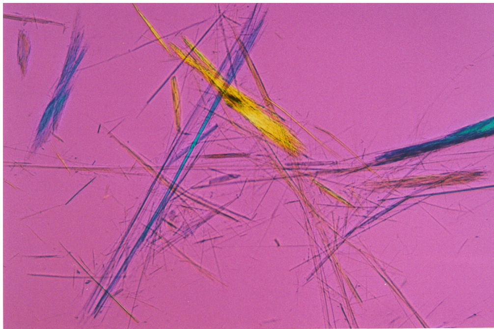
Figure 13. PLM Micrograph of Asbestos Fiber Bundles From Libby Vermiculite
