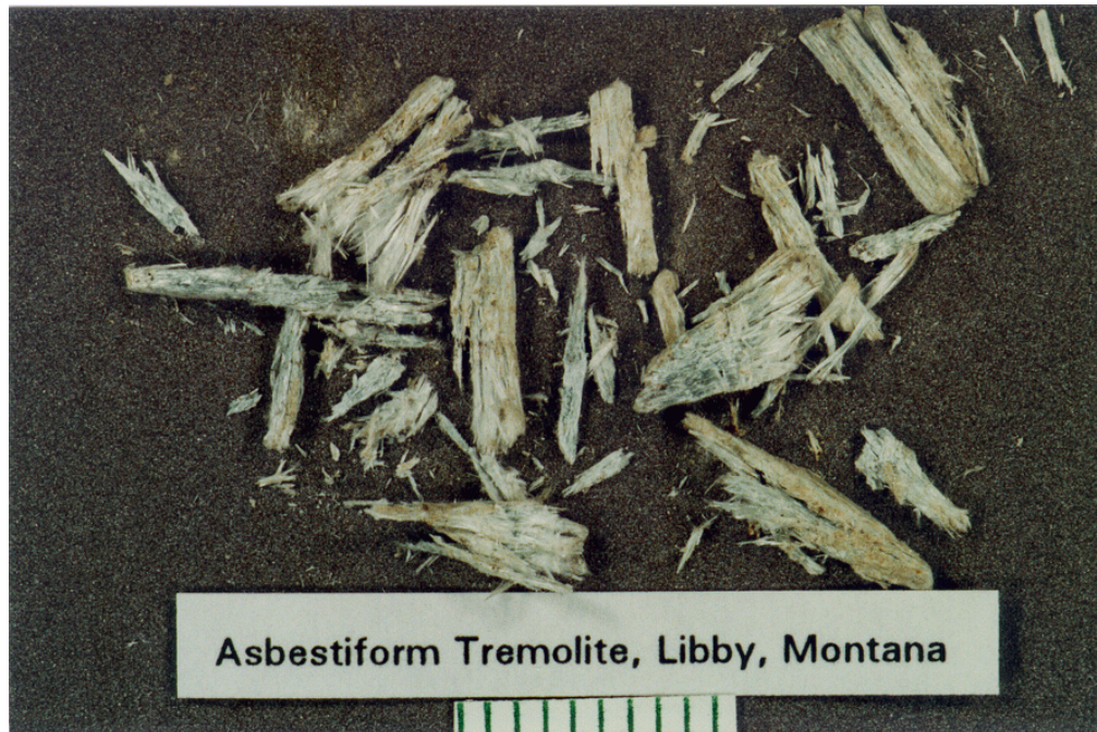
Figure 12. Asbestos Fiber Bundles Picked From Libby Vermiculite (Formerly Called Tremolite, Now Called Richterite)
