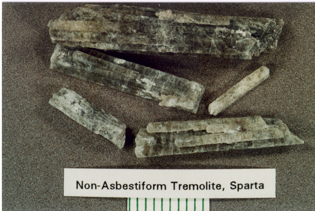
Figure 10. Non-Asbestiform Tremolite, Sparta, New Jersey
